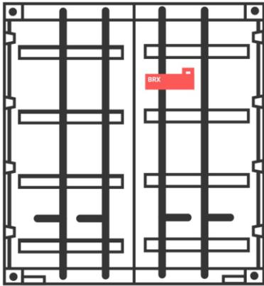
Intermodal smart barrier lock, build from Heavy Duty steel housing, 15-20 Year battery life without a single charge able to lock/unlock the door: 1) remotely, 2) via mobile app, 3) geofencing, or 4) Machine Learning
