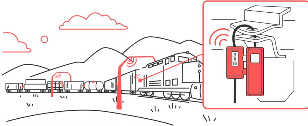
Active Bluetooth, Tamper-Resistant, Cable cut detection, which communicates with Red Flag readers with a range up to 200 meters at speeds topping 70MPH.
