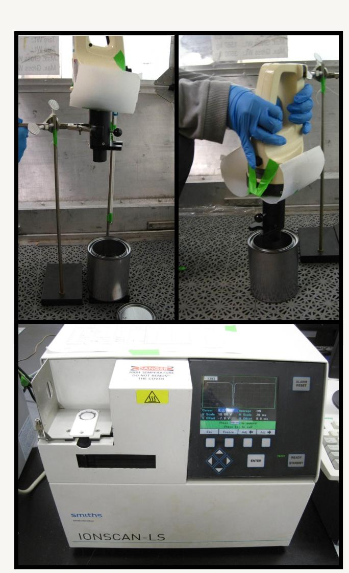
Dynamic PSPME sampling at different distances (top) followed by detection using commercial IMS (Smiths IONSCAN-LS).
