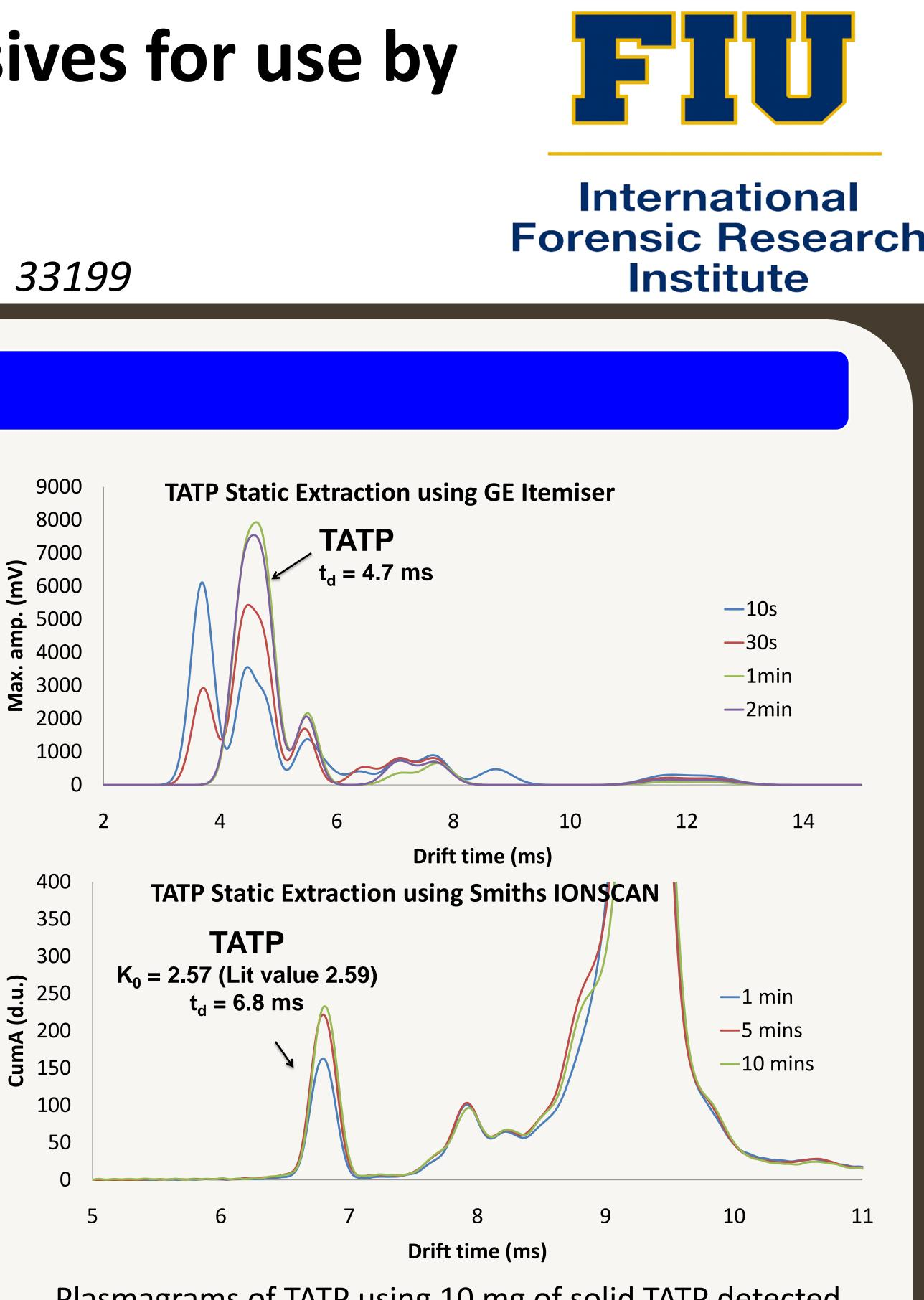
Plasmagrams of TATP using 10 mg of solid TATP detected by GE Itemizer (top) and 0.5 µg of liquid standard TATP detected by Smiths IONSCAN-LS (bottom).
