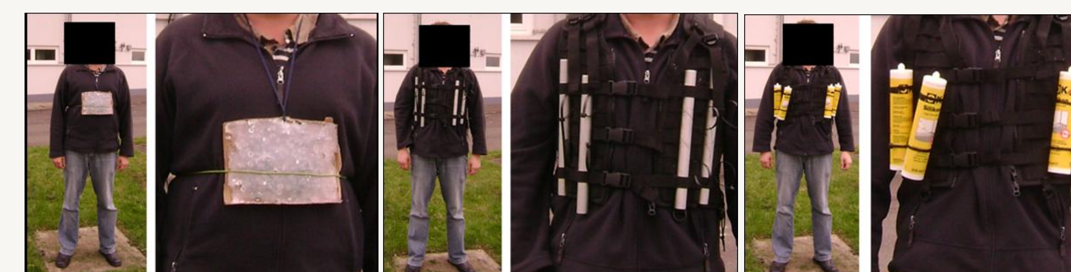
Figure 2: image of the target with different threats (a) a silicon metallic object on the chest (b) metallic pipes on the chest (c) silicon pipes on the chest.
