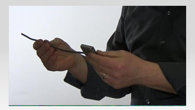
Cable is twisted and pulled at the same time. The cable can be removed and later reinserted without evidence
