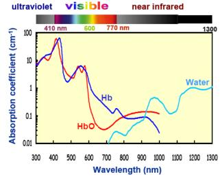
By measuring absorptions at multiple wavelengths, one can calculate the concentrations of the chromophores
