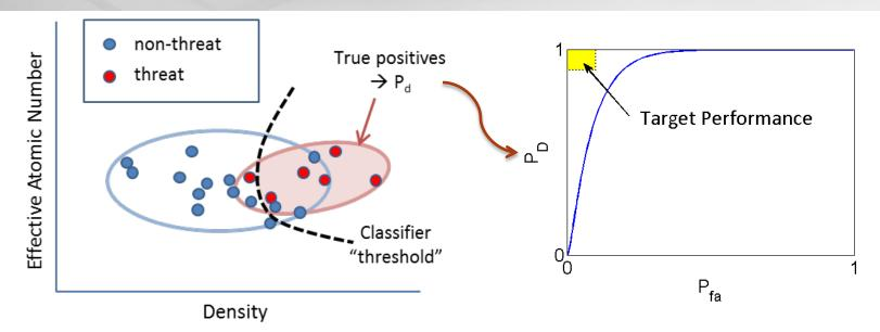
Increasing separation via complementary ("orthogonal") technology
