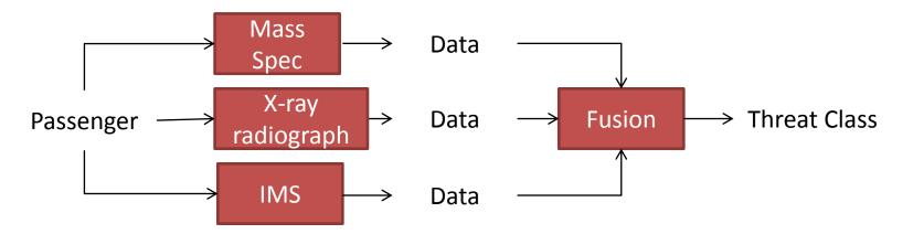
A fusion algorithm is only as good as the sensors it relies on. A single failed sensor can introduce a large amount of risk to an otherwise operational system.
