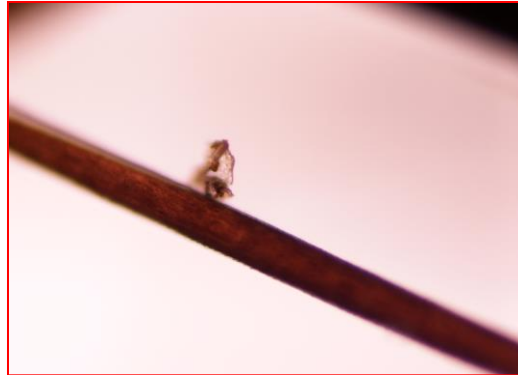
Particle of explosive on hair observed under magnification
