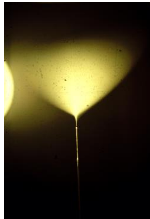
Dense Droplet Mist From Taylor Cone Back-lit Photograph
