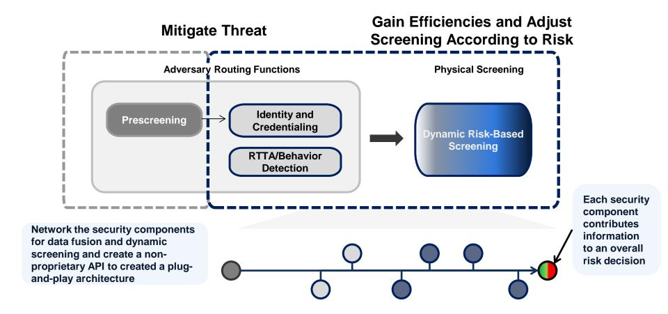
Introduce an API and IT architecture which allows for a) data persistence, b) data fusion, and c) dynamic physical screening based on risk. *These foundational elements will enable the emergence of Dynamic Risk Based Screening*.
