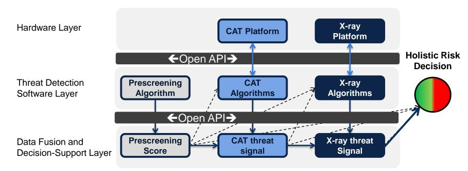
The D-RBS architecture utilizes a common API to enable different logical layers of the system to communicate and dynamically screen passengers in real time. Data from multiple sources inform each successive step in the process, as well as the final risk decision.
