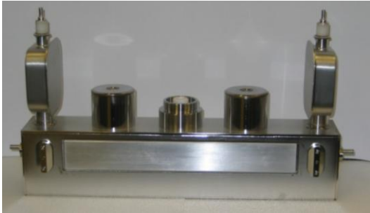
Linear multibeam tube for 3D mammography
