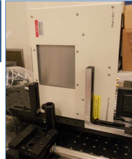
Detector: Shad- o-box 4k; 10 cm active area, 50 \mu\text{m} pixel size
