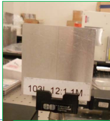
Grid, held in mount with set screws
