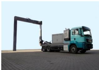
TUDOR Scan ML64 Robotic trucks scanners based on dual energy LINAC technology
