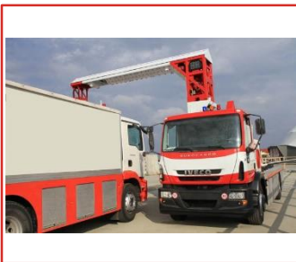
TUDOR Scan 1MC Robotic trucks scanners based on dual energy Gamma technology
