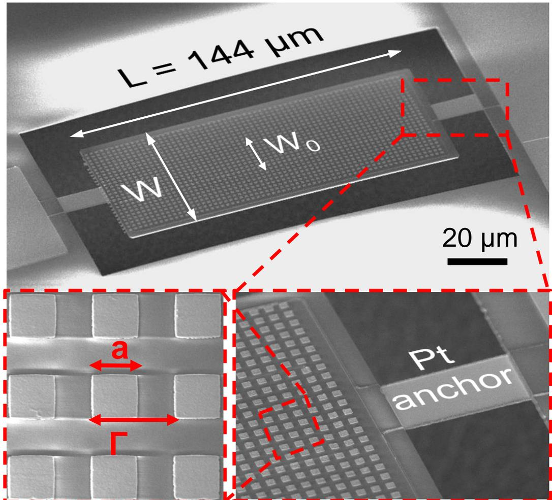
$a = 1.2$  or  $1.3 \mu\text{m}$ ,  $\Gamma = 2.2 \mu\text{m}$ ,  $W = 60 \mu\text{m}$ ,  $W_0 = 20 \mu\text{m}$
