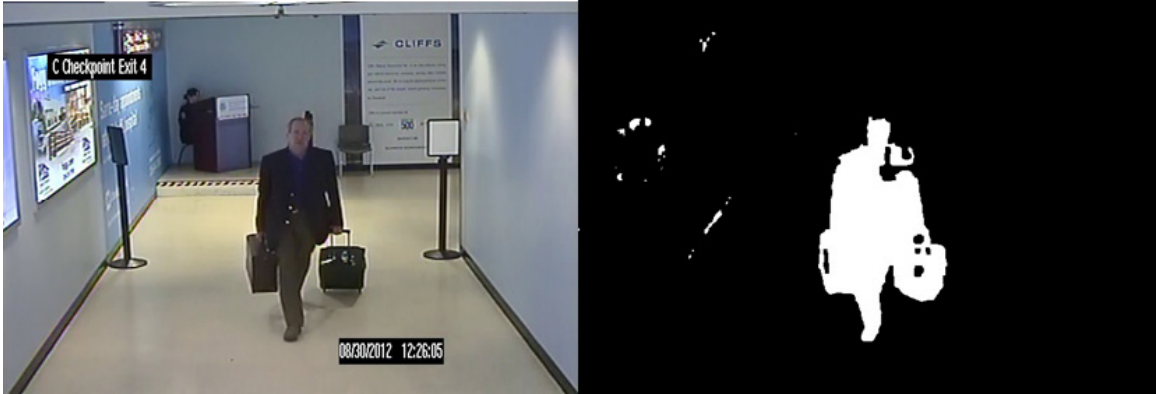
Figure 3.5: Camera video frame (left) with MOG Background subtraction results (right). White indicates foreground region.
