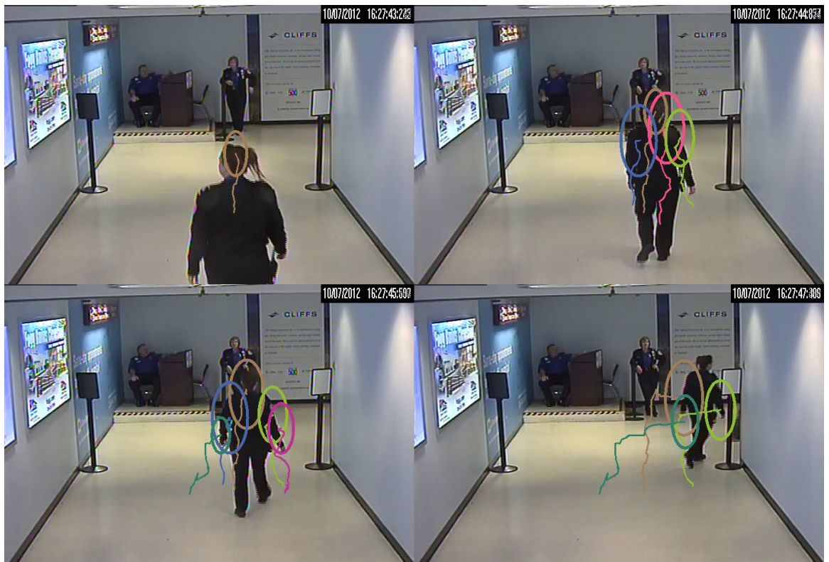
Figure 3.14: Example of smart adapting of target size and position over time using background subtraction output.
