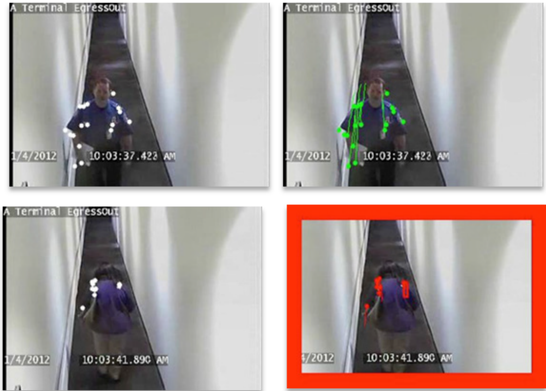
Figure 3.8: Corner Tracklets. Detected corners are tracked (left) and then used to identify counter-flow (right).
