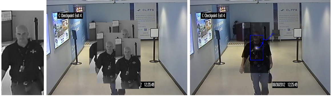
Figure 3.7: Pedestrian tracked using circulant tracker. Cross-correlation with a target template (left) is used to search possible locations (center). The correct location (right) is indicated by maximum of cross-correlation result.
