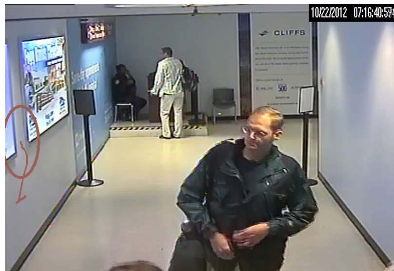
Figure 4.3: False alarm caused by incorrect detection and tracking using the single camera smart foreground blob tracking approach (see 3.3.3.1)
