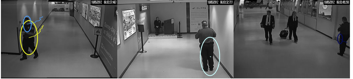
Figure 3.10: Counter-flow Detection using the two primary cameras (left & center) with one verify camera (right) approach.
