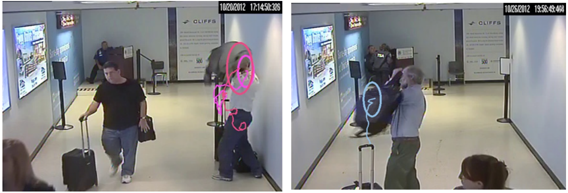
Figure 4.2: False alarm caused by passenger lifting luggage using the single camera smart foreground blob tracking approach (see 3.3.3.1)
