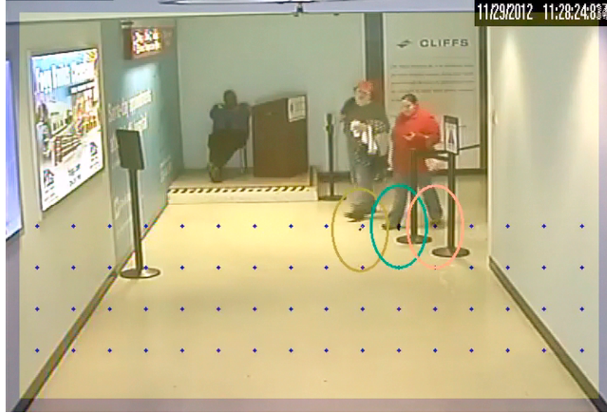
Figure 3.6: Over-Tracking Target Initialization. Camera video frame showing locations where trackers will be initialized.
