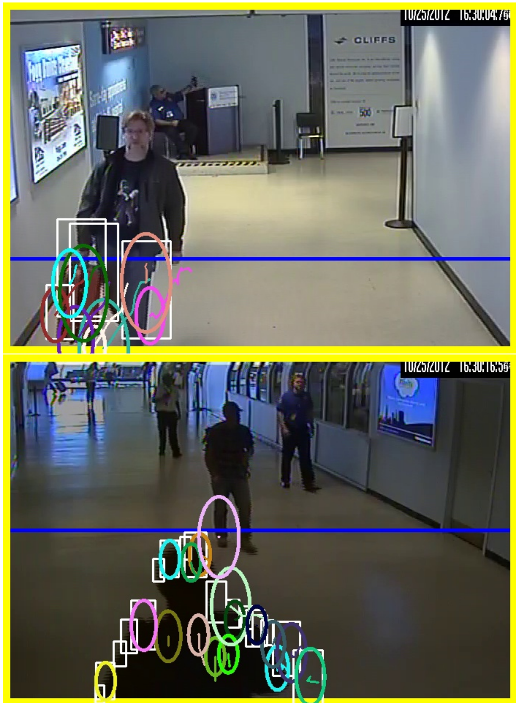
Figure 3.4: Targets are initialization when foreground is detected below the blue line. Colored ellipses indicates an active target. The white rectangles indicate newly detected foreground regions.
