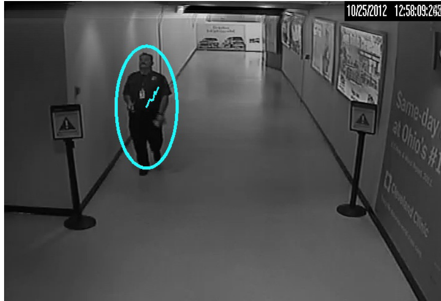
Figure 3.3: Detected pedestrian using HOG features
